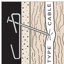
**Behind the Walls.** The nail from a picture hanger or flooring can actually puncture insulation and cause arcing.
