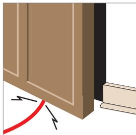
**Damaged Cords.** Insulation can be damaged when furniture is pushed up against a cord or it becomes caught and pinched in a door.
