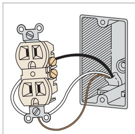
**Loose Connections.** A wall plug or switch can cause an electrical fault if not properly installed, or if the connections have become loose.
